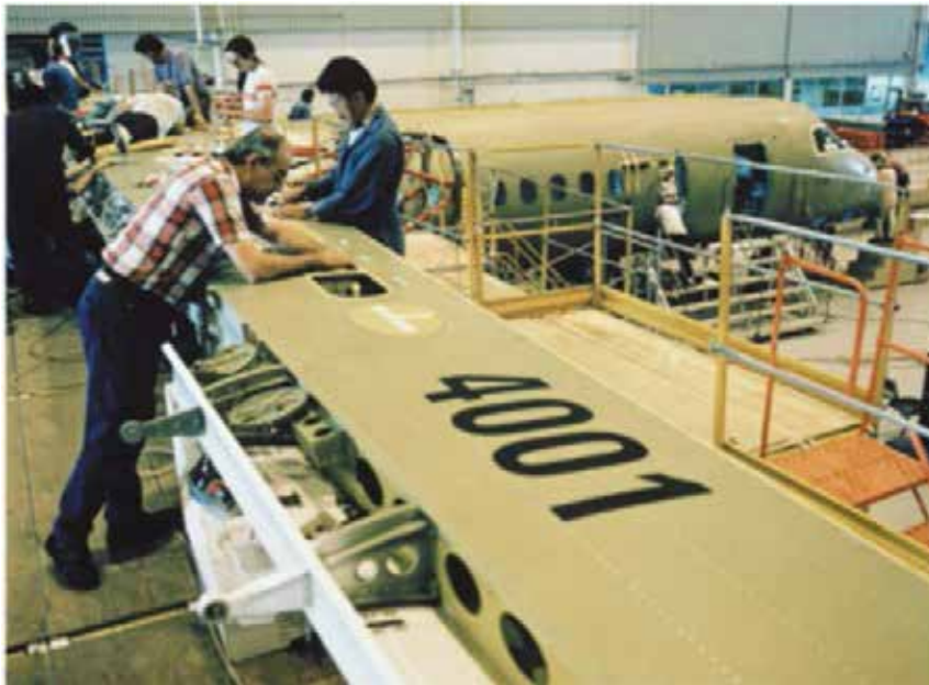
Figure A-5 Bombardier QR 400 Wing Assembly
