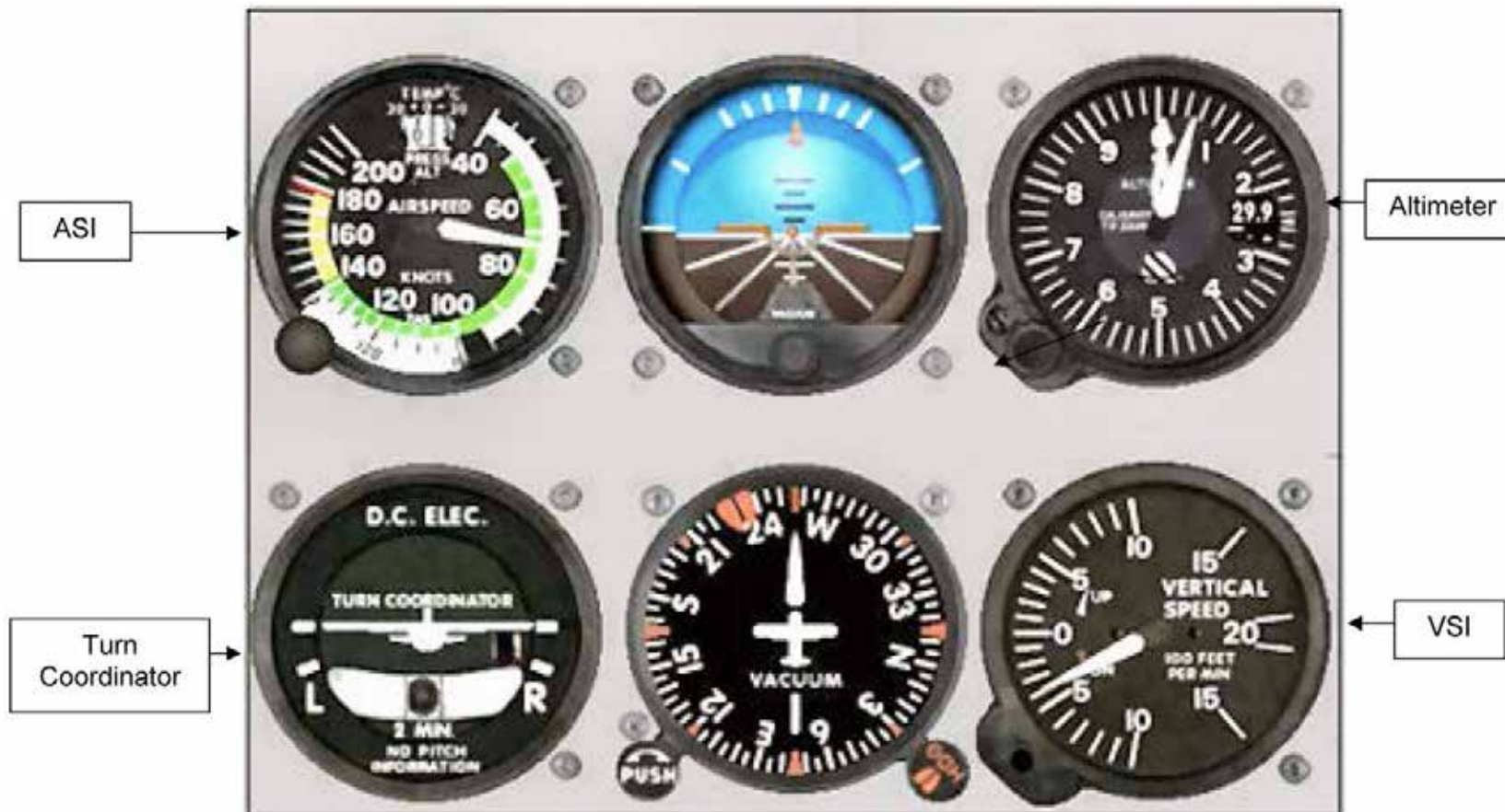
Figure A-1 Cessna Flight Instrument Panel
