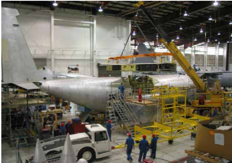
Figure A-1 Rebuilding a C-130 Centre Wing
