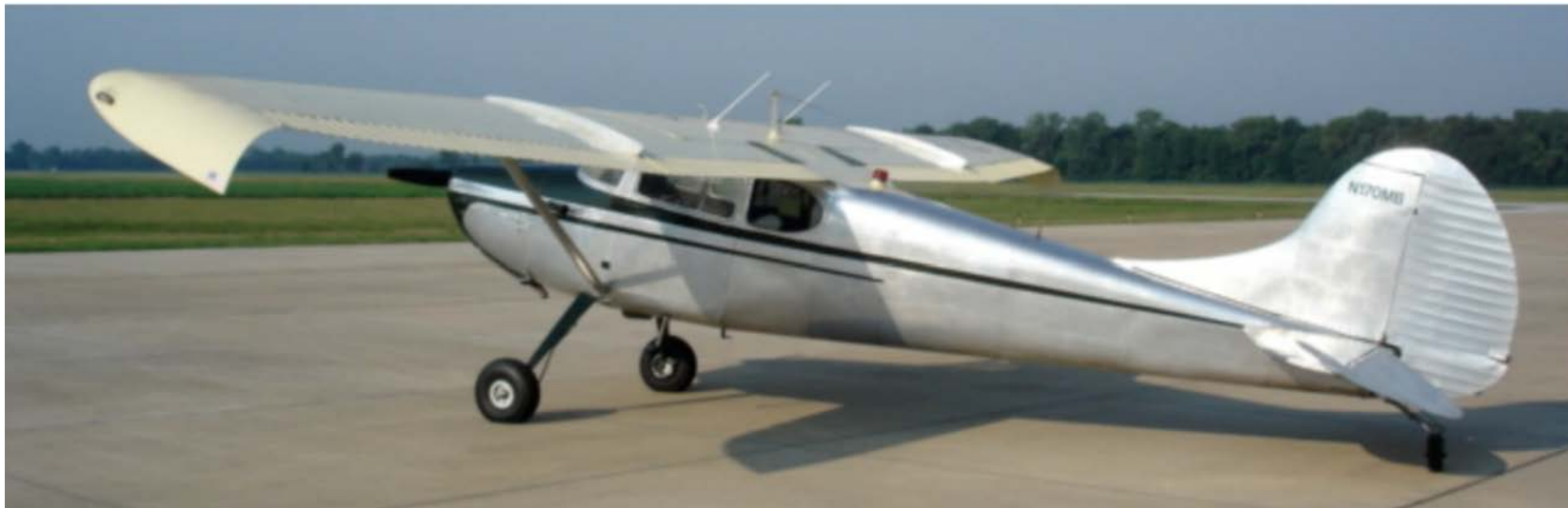
Figure A-8 Drooping the Wing Tips
