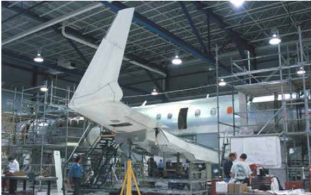
Figure A-11 Bombardier CRJ700 Assembly
