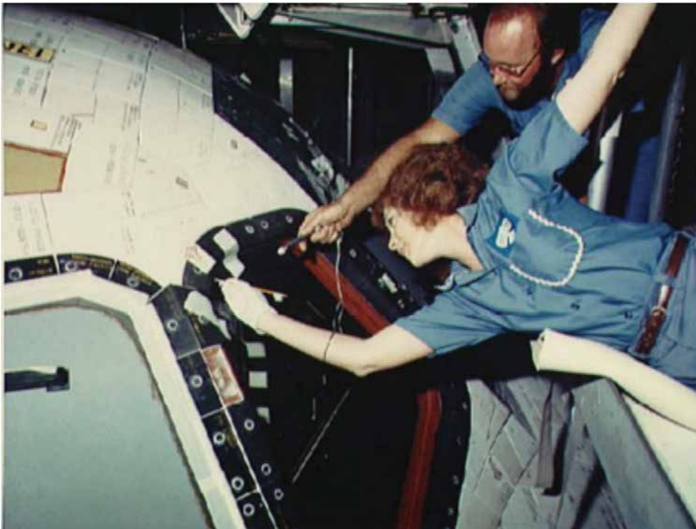
Figure B-3 Repairing TPS on Columbia
