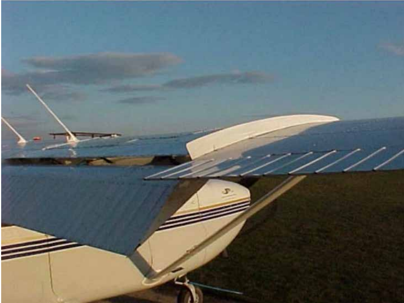
Figure A-9 Wing Fences
