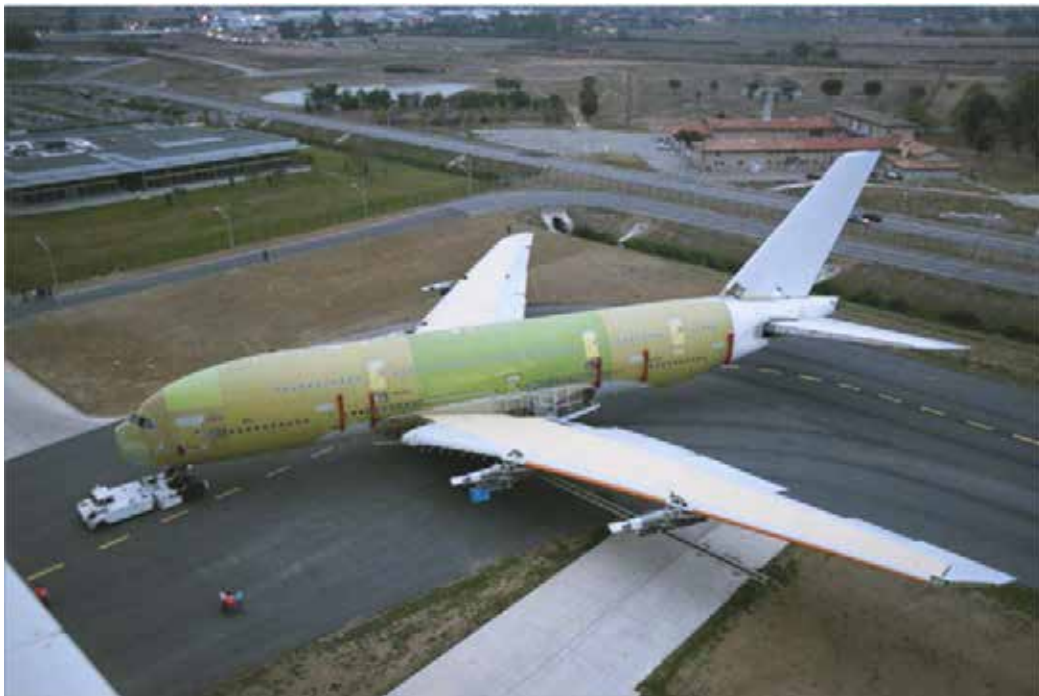
Figure B-4 Empty Pylons
