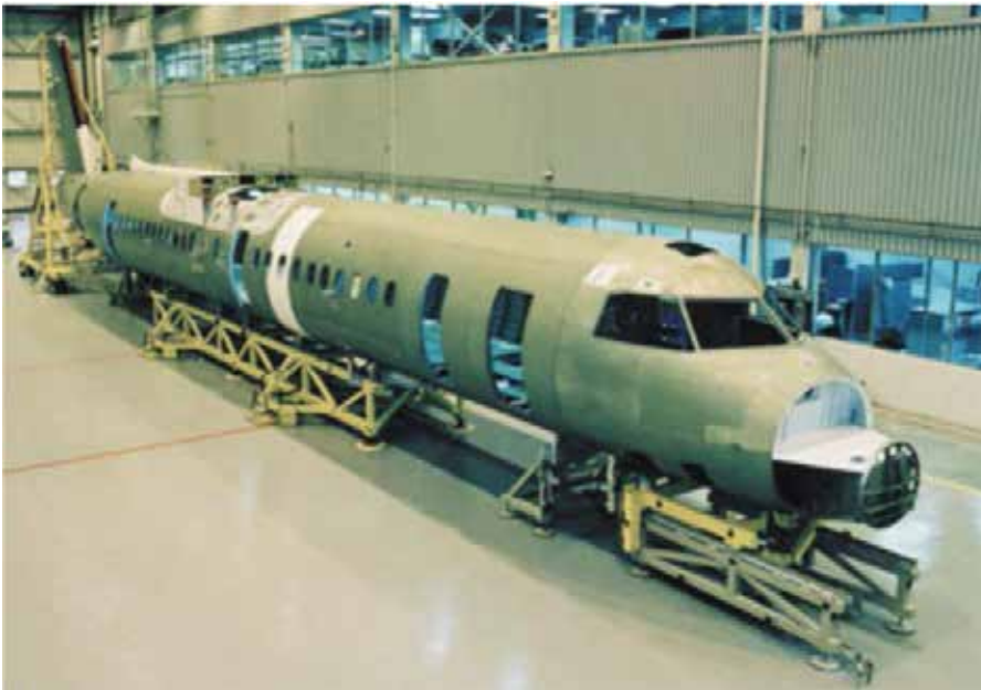
Figure A-4 Bombardier QR 400 Fuselage Assembly
