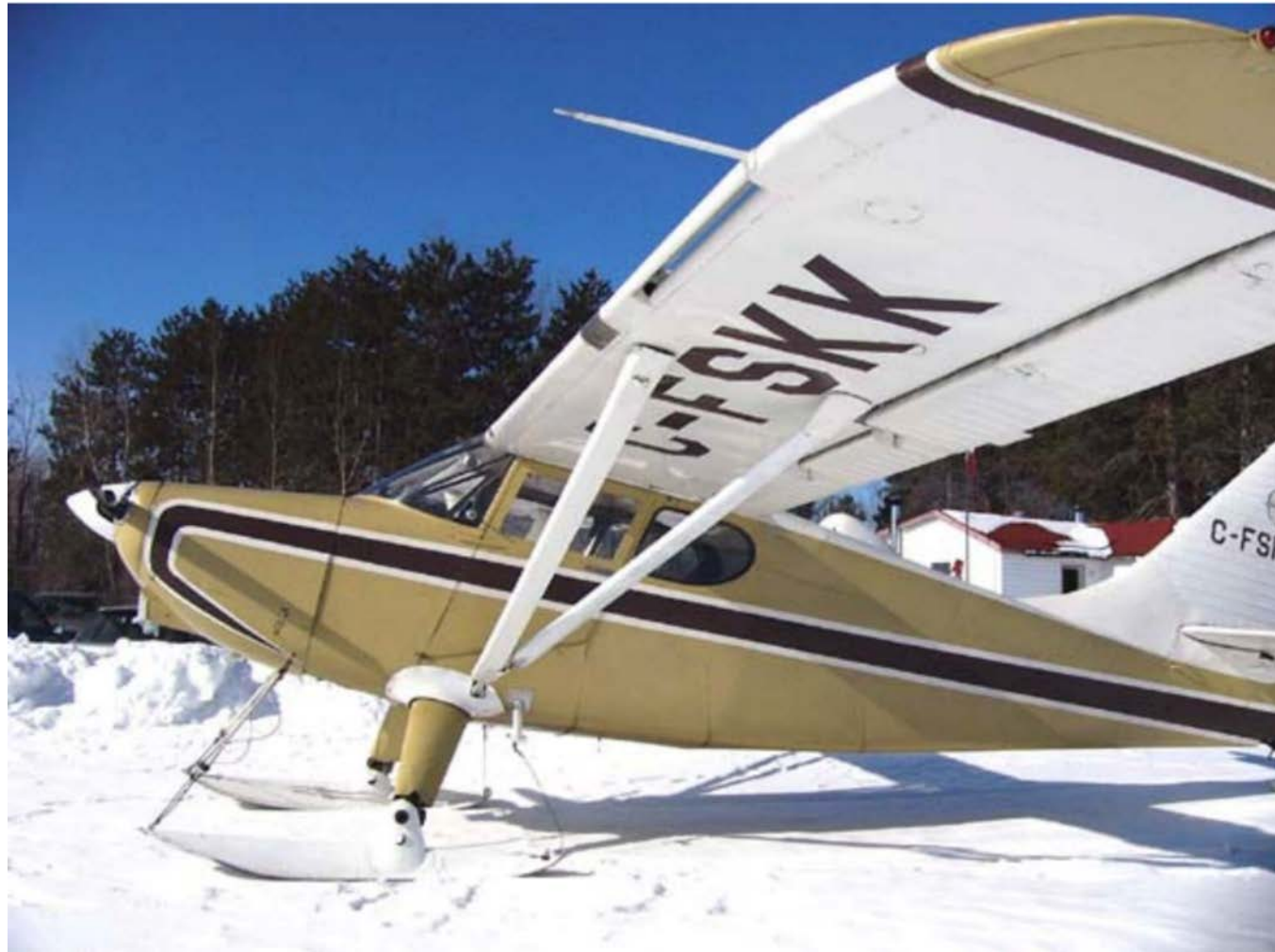
Figure A-11 Leading Edge Slot
